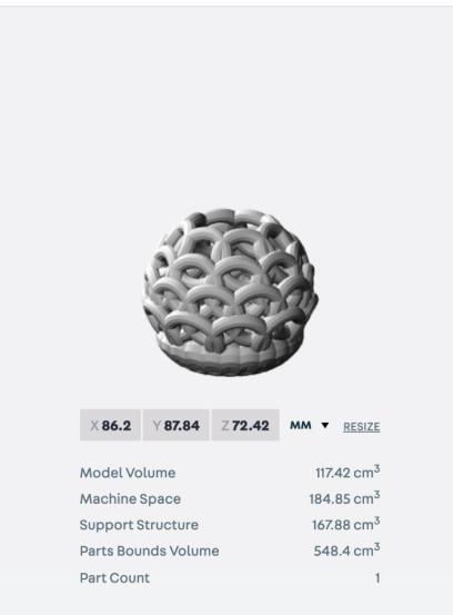
The screenshot shows a 3D model of a spherical lampshade with a complex, woven texture. On the left, there are coordinate values (X 86.2, Y 87.84, Z 72.42) and a 'RESIZE' button. Below the model are technical specifications: Model Volume (117.42 cm³), Machine Space (184.85 cm³), Support Structure (167.88 cm³), Parts Bounds Volume (548.4 cm³), and Part Count (1).
