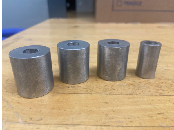
Spacers Between Ground Plate and Game Board
